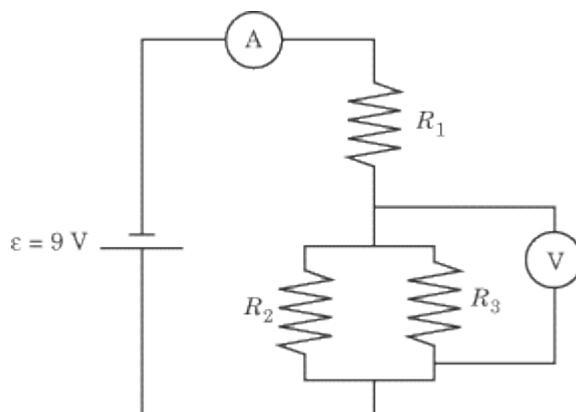
In the diagram above,  $\mathcal{E} = 9 \text{ V}$ ,  $R_1 = 5 \Omega$ ,  $R_2 = 5 \Omega$ , and  $R_3 = 20 \Omega$ . What are the values measured by the ammeter and the voltmeter?
