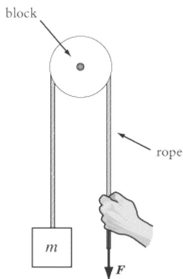
**Pulleys** are simple machines that consist of a rope that slides around a disk, called a pulley. Their main function is to change the direction of the tension force in a rope. The pulley systems that appear on SAT II Physics almost always consist of idealized, massless and frictionless pulleys, and idealized ropes that are massless and that don't stretch. These somewhat unrealistic parameters mean that:
