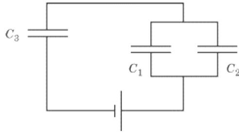
Given  $C_1 = 2 \text{ } \hat{\text{A}}\mu\text{F}$ ,  $C_2 = 6 \text{ } \hat{\text{A}}\mu\text{F}$ , and  $C_3 = 3 \text{ } \hat{\text{A}}\mu\text{F}$ , what is the total capacitance of the circuit in the figure above?
