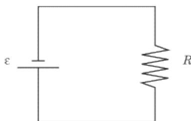
Zigzags represent resistors, and a pair of parallel, unequal lines represents a battery cell. The longer line is the positive terminal and the shorter line is the negative terminal. That means the current flows from the longer line around the circuit to the shorter line. In the diagram above, the current flows counterclockwise. Often, more than one set of unequal parallel lines are arranged together; this just signifies a number of battery cells arranged in series.
