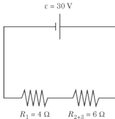
1. **Treating the equivalent resistance of the resistors in parallel as a single resistor, calculate the total resistance by adding resistors in series.** The diagram above gives us two resistors in series. Calculating the total resistance of the circuit couldn't be easier:
