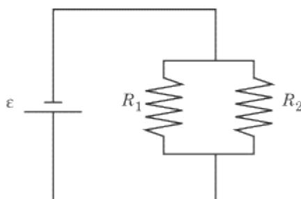
In this circumstance, it is often useful to calculate the equivalent resistance as if there were only one resistor, rather than deal with each resistor individually. Calculating the equivalent resistance of two or more resistors in parallel is a little more complicated than calculating the total resistance of two or more resistors in series. Given two resistors,  $R_1$  and  $R_2$ , in parallel, the equivalent resistance,  $R_t$ , is:
