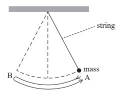
The equation for a simple pendulum is  $T = 2\pi \sqrt{\frac{l}{g}}$
