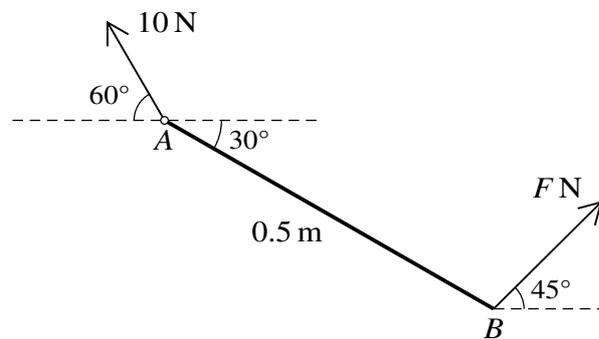
A non-uniform rod  $AB$  of length 0.5 m is freely hinged to a fixed point  $A$ . The rod is in equilibrium at an angle of  $30^\circ$  with the horizontal with  $B$  below the level of  $A$ . Equilibrium is maintained by a force of magnitude  $F$  N applied at  $B$  acting at  $45^\circ$  above the horizontal in the vertical plane containing  $AB$ . The force exerted by the hinge on the rod has magnitude 10 N and acts at an angle of  $60^\circ$  above the horizontal (see diagram).
