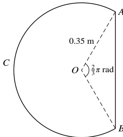
A uniform lamina  $ABC$  is in the form of a major segment of a circle with centre  $O$  and radius  $0.35 \text{ m}$ . The straight edge of the lamina is  $AB$ , and angle  $AOB = \frac{2}{3}\pi$  radians (see diagram).
