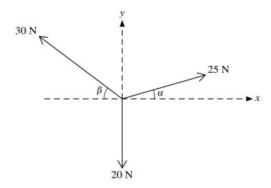
Three coplanar forces act at a point. The magnitudes of the forces are 20 N, 25 N and 30 N, and the directions in which the forces act are as shown in the diagram, where  $\sin \alpha = 0.28$  and  $\cos \alpha = 0.96$ , and  $\sin \beta = 0.6$  and  $\cos \beta = 0.8$ .
