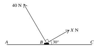
Forces of magnitude X N and 40 N act on a block B of mass 15 kg, which is in equilibrium in contact with a horizontal surface between points A and C on the surface. The forces act in the same vertical plane and in the directions shown in the diagram.
