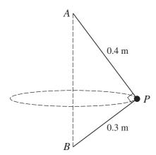
A particle P of mass 0.2 kg is attached to a fixed point A by a light inextensible string of length 0.4 m. A second light inextensible string of length 0.3 m connects P to a fixed point B which is vertically below A. The particle P moves in a horizontal circle, which has its centre on the line AB, with the angle  $APB = 90^{\circ}$  (see diagram).
