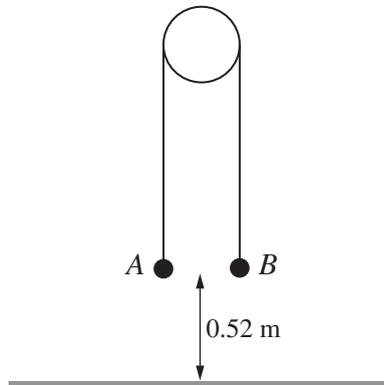
Particles  $A$  and  $B$ , of masses 0.3 kg and 0.7 kg respectively, are attached to the ends of a light inextensible string. The string passes over a fixed smooth pulley.  $A$  is held at rest and  $B$  hangs freely, with both straight parts of the string vertical and both particles at a height of 0.52 m above the floor (see diagram).  $A$  is released and both particles start to move.
