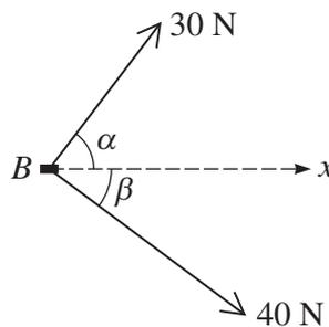
A block  $B$  lies on a rough horizontal plane. Horizontal forces of magnitudes  $30 \text{ N}$  and  $40 \text{ N}$ , making angles of  $\alpha$  and  $\beta$  respectively with the  $x$ -direction, act on  $B$  as shown in the diagram, and  $B$  is moving in the  $x$ -direction with constant speed. It is given that  $\cos \alpha = 0.6$  and  $\cos \beta = 0.8$ .
