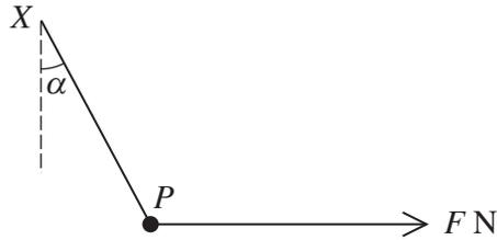
A particle  $P$  of mass  $0.3 \text{ kg}$  is attached to one end of a light inextensible string. The other end of the string is attached to a fixed point  $X$ . A horizontal force of magnitude  $F \text{ N}$  is applied to the particle, which is in equilibrium when the string is at an angle  $\alpha$  to the vertical, where  $\tan \alpha = \frac{8}{15}$  (see diagram). Find the tension in the string and the value of  $F$ . [4]
