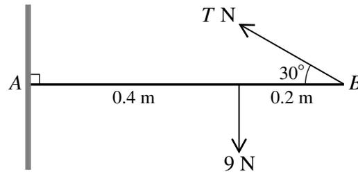
A non-uniform rod  $AB$ , of length  $0.6\text{ m}$  and weight  $9\text{ N}$ , has its centre of mass  $0.4\text{ m}$  from  $A$ . The end  $A$  of the rod is in contact with a rough vertical wall. The rod is held in equilibrium, perpendicular to the wall, by means of a light string attached to  $B$ . The string is inclined at  $30^\circ$  to the horizontal. The tension in the string is  $T\text{ N}$  (see diagram).
