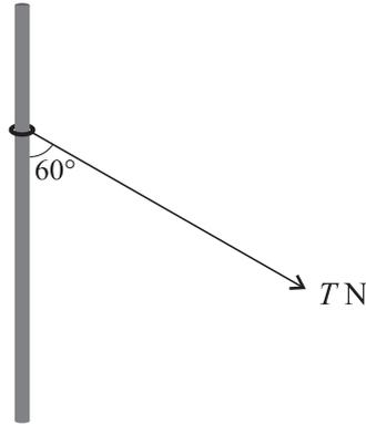
A ring of mass 4 kg is threaded on a fixed rough vertical rod. A light string is attached to the ring, and is pulled with a force of magnitude  $T$  N acting at an angle of  $60^\circ$  to the downward vertical (see diagram). The ring is in equilibrium.
