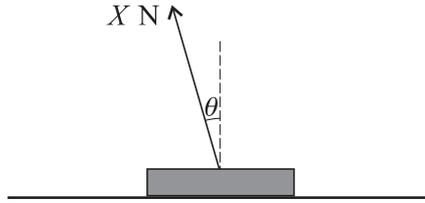
A stone slab of mass 320 kg rests in equilibrium on rough horizontal ground. A force of magnitude  $X$  N acts upwards on the slab at an angle of  $\theta$  to the vertical, where  $\tan \theta = \frac{7}{24}$  (see diagram).
