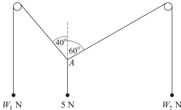
Each of three light strings has a particle attached to one of its ends. The other ends of the strings are tied together at a point  $A$ . The strings are in equilibrium with two of them passing over fixed smooth horizontal pegs, and with the particles hanging freely. The weights of the particles, and the angles between the sloping parts of the strings and the vertical, are as shown in the diagram. Find the values of  $W_1$  and  $W_2$ .
