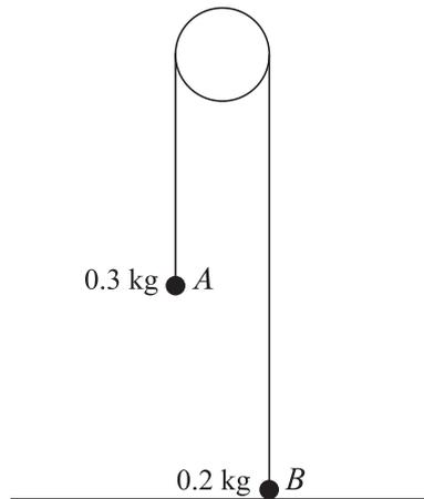
Two particles  $A$  and  $B$ , of masses  $0.3 \text{ kg}$  and  $0.2 \text{ kg}$  respectively, are attached to the ends of a light inextensible string which passes over a smooth fixed pulley. Particle  $B$  is held on the horizontal floor and particle  $A$  hangs in equilibrium. Particle  $B$  is released and each particle starts to move vertically with constant acceleration of magnitude  $a \text{ m s}^{-2}$ .
