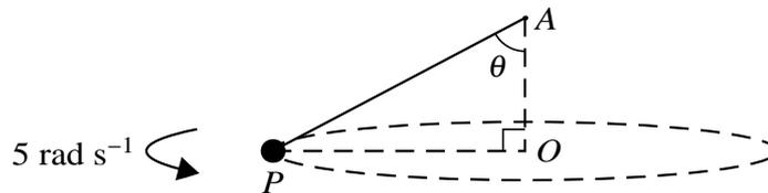
One end of a light inextensible string is attached to a fixed point  $A$  and the other end of the string is attached to a particle  $P$ . The particle  $P$  moves with constant angular speed  $5 \text{ rad s}^{-1}$  in a horizontal circle which has its centre  $O$  vertically below  $A$ . The string makes an angle  $\theta$  with the vertical (see diagram). The tension in the string is three times the weight of  $P$ .
