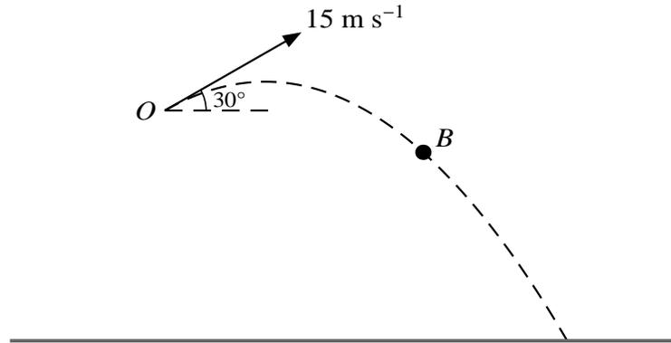
A small ball  $B$  is projected from a point  $O$  above horizontal ground, with initial speed  $15 \text{ m s}^{-1}$  at an angle of projection of  $30^\circ$  above the horizontal (see diagram). The ball strikes the ground  $3 \text{ s}$  after projection.
