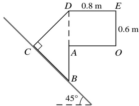
The diagram shows the cross-section  $OABCDE$  through the centre of mass of a uniform prism on a rough inclined plane. The portion  $ADEO$  is a rectangle in which  $AD = OE = 0.6\text{ m}$  and  $DE = AO = 0.8\text{ m}$ ; the portion  $BCD$  is an isosceles triangle in which angle  $BCD$  is a right angle, and  $A$  is the mid-point of  $BD$ . The plane is inclined at  $45^\circ$  to the horizontal,  $BC$  lies along a line of greatest slope of the plane and  $DE$  is horizontal.
