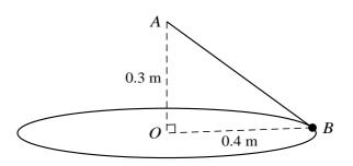
A small bead *B* of mass *m* kg moves with constant speed in a horizontal circle on a fixed smooth wire. The wire is in the form of a circle with centre *O* and radius 0.4 m. One end of a light elastic string of natural length 0.4 m and modulus of elasticity 42m N is attached to *B*. The other end of the string is attached to a fixed point *A* which is 0.3 m vertically above *O* (see diagram).
