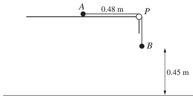
Particle  $A$  of mass 1.26 kg and particle  $B$  of mass 0.9 kg are attached to the ends of a light inextensible string. The string passes over a small smooth pulley  $P$  which is fixed at the edge of a rough horizontal table.  $A$  is held at rest at a point 0.48 m from  $P$ , and  $B$  hangs vertically below  $P$ , at a height of 0.45 m above the floor (see diagram). The coefficient of friction between  $A$  and the table is  $\frac{2}{7}$ .  $A$  is released and the particles start to move.
