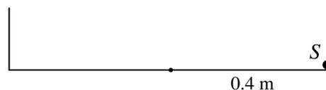
A small sphere  $S$  of mass  $m \text{ kg}$  is moving inside a fixed smooth hollow cylinder whose axis is vertical.  $S$  moves with constant speed in a horizontal circle of radius  $0.4 \text{ m}$  and is in contact with both the plane base and the curved surface of the cylinder (see diagram).
