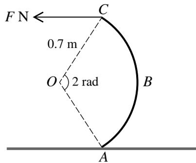
The diagram shows a uniform object  $ABC$  of weight  $3 \text{ N}$  in the form of an arc of a circle with centre  $O$  and radius  $0.7 \text{ m}$ . The angle  $AOC$  is  $2 \text{ radians}$ . The object rests in equilibrium with  $A$  on a horizontal surface and  $C$  vertically above  $A$ . Equilibrium is maintained by a horizontal force of magnitude  $F \text{ N}$  applied at  $C$  in the plane of the object. Calculate  $F$ . [4]
