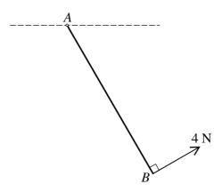
A uniform rod AB of weight 16 N is freely hinged at A to a fixed point. A force of magnitude 4 N acting perpendicular to the rod is applied at B (see diagram). Given that the rod is in equilibrium,
