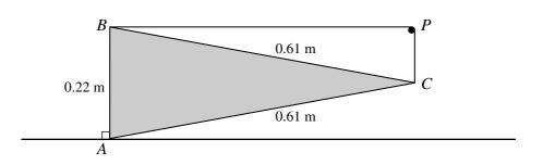
*ABC* is a uniform triangular lamina of weight 19 N, with AB = 0.22 m and AC = BC = 0.61 m. The plane of the lamina is vertical. A rests on a rough horizontal surface, and AB is vertical. The equilibrium of the lamina is maintained by a light elastic string of natural length 0.7 m which passes over a small smooth peg P and is attached to B and C. The portion of the string attached to B is horizontal, and the portion of the string attached to C is vertical (see diagram).
