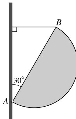
$AB$  is the diameter of a uniform semicircular lamina which has radius 0.3 m and mass 0.4 kg. The lamina is hinged to a vertical wall at  $A$  with  $AB$  inclined at  $30^\circ$  to the vertical. One end of a light inextensible string is attached to the lamina at  $B$  and the other end of the string is attached to the wall vertically above  $A$ . The lamina is in equilibrium in a vertical plane perpendicular to the wall with the string horizontal (see diagram).
