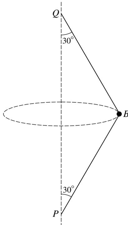
A small ball  $B$  of mass  $0.4 \text{ kg}$  is attached to fixed points  $P$  and  $Q$  on a vertical axis by two light inextensible strings of equal length. Both strings are taut and each is inclined at  $30^\circ$  to the vertical. The ball moves in a horizontal circle (see diagram).
