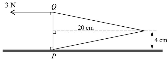
A uniform solid cone has height 20 cm and base radius 4 cm.  $PQ$  is a diameter of the base of the cone. The cone is held in equilibrium, with  $P$  in contact with a horizontal surface and  $PQ$  vertical, by a force applied at  $Q$ . This force has magnitude 3 N and acts parallel to the axis of the cone (see diagram). Calculate the mass of the cone. [4]
