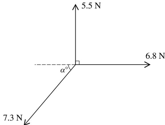
Three coplanar forces act at a point. The magnitudes of the forces are 5.5 N, 6.8 N and 7.3 N, and the directions in which the forces act are as shown in the diagram. Given that the resultant of the three forces is in the same direction as the force of magnitude 6.8 N, find the value of  $\alpha$  and the magnitude of the resultant. [4]
