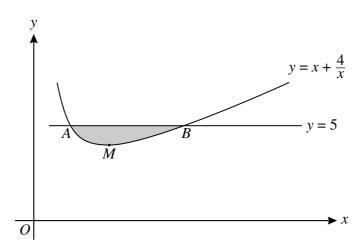
The diagram shows part of the curve  $y = x + \frac{4}{x}$  which has a minimum point at M. The line y = 5 intersects the curve at the points A and B.
