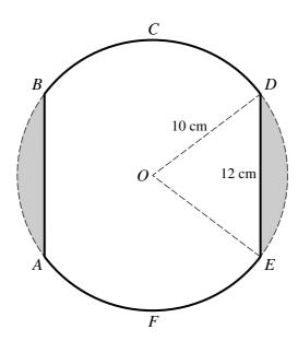
The diagram shows a metal plate ABCDEF which has been made by removing the two shaded regions from a circle of radius 10 cm and centre O. The parallel edges AB and ED are both of length 12 cm.
