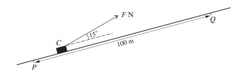
A crate C is pulled at constant speed up a straight inclined path by a constant force of magnitude F N, acting upwards at an angle of  $15^{\circ}$  to the path. C passes through points P and Q which are 100 m apart (see diagram). As C travels from P to Q the work done against the resistance to C's motion is 900 J, and the gain in C's potential energy is 2100 J. Write down the work done by the pulling force as C travels from P to Q, and hence find the value of F.
