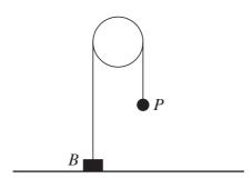
A block B of mass 5 kg is attached to one end of a light inextensible string. A particle P of mass 4 kg is attached to other end of the string. The string passes over a smooth pulley. The system is in equilibrium with the string taut and its straight parts vertical. B is at rest on the ground (see diagram). State the tension in the string and find the force exerted on B by the ground.
