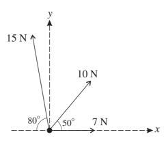
Forces of magnitudes 7 N, 10 N and 15 N act on a particle in the directions shown in the diagram.
