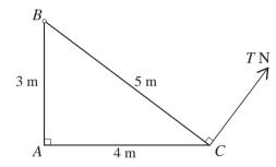
Uniform rods *AB*, *AC* and *BC* have lengths 3 m, 4 m and 5 m respectively, and weights 15 N, 20 N and 25 N respectively. The rods are rigidly joined to form a right-angled triangular frame *ABC*. The frame is hinged at *B* to a fixed point and is held in equilibrium, with *AC* horizontal, by means of an inextensible string attached at *C*. The string is at right angles to *BC* and the tension in the string is *T* N (see diagram).
