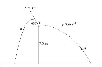
Particles *A* and *B* are projected simultaneously from the top *T* of a vertical tower, and move in the same vertical plane. *T* is 7.2 m above horizontal ground. *A* is projected horizontally with speed  $8 \text{ m s}^{-1}$  and *B* is projected at an angle of  $60^{\circ}$  above the horizontal with speed  $5 \text{ m s}^{-1}$ . *A* and *B* move away from each other (see diagram).
