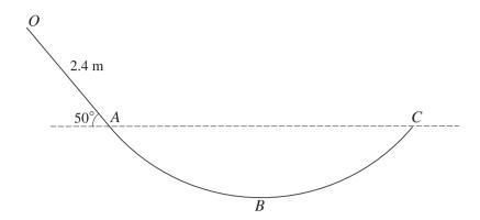
OABC is a vertical cross-section of a smooth surface. The straight part OA has length 2.4 m and makes an angle of  $50^{\circ}$  with the horizontal. A and C are at the same horizontal level and B is the lowest point of the cross-section (see diagram). A particle P of mass 0.8 kg is released from rest at O and moves on the surface. P remains in contact with the surface until it leaves the surface at C. Find
