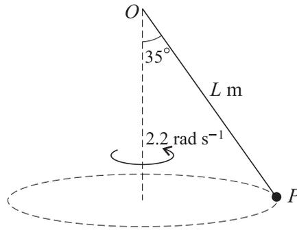
A particle  $P$  of mass  $m$  kg is attached to one end of a light inextensible string of length  $L$  m. The other end of the string is attached to a fixed point  $O$ . The particle  $P$  moves with constant speed in a horizontal circle, with the string taut and inclined at  $35^\circ$  to the vertical.  $OP$  rotates with angular speed  $2.2 \text{ rad s}^{-1}$  about the vertical axis through  $O$  (see diagram). Find
