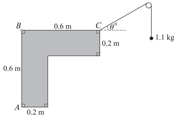
A uniform lamina of weight  $15 \text{ N}$  has dimensions as shown in the diagram.
