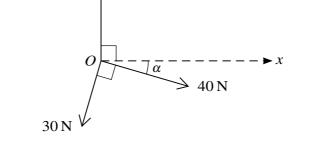
Coplanar forces of magnitudes 50 N, 40 N and 30 N act at a point *O* in the directions shown in the diagram, where  $\tan \alpha = \frac{7}{24}$ .
