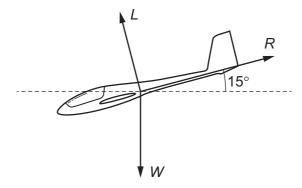
Which vector triangle could represent the forces acting on the glider?
