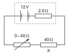
The resistance of the variable resistor is changed from 0 to 40  $\Omega$ .
