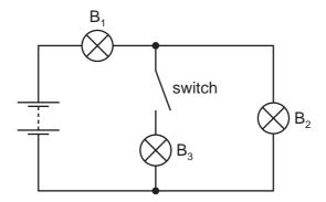
Initially the switch is closed. The switch is then opened and lamp B<sub>3</sub> goes out.
