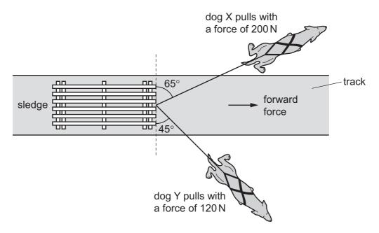
Dog X pulls with a force of  $200\,\text{N}$  at an angle of  $65^\circ$  to the front edge of the sledge. Dog Y pulls with a force of  $120\,\text{N}$  at an angle of  $45^\circ$  to the front edge of the sledge.
