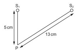
The sources each generate a wave of wavelength 2.0 cm. Each source produces a wave that has amplitude  $x_0$  when it reaches point P.
