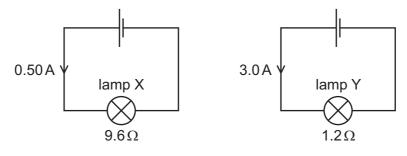
What is the ratio  $\frac{\text{power in lamp X}}{\text{power in lamp Y}}$
