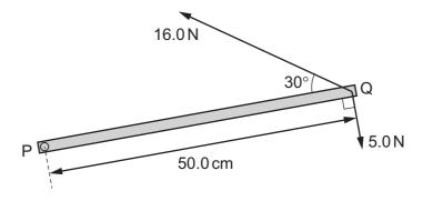
Two forces of 16.0 N and 5.0 N are in the horizontal plane and act on end Q as shown in the diagram.
