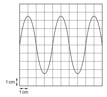
The oscilloscope time-base setting is 0.5 ms cm<sup>-1</sup> and the Y-plate sensitivity is 2 V cm<sup>-1</sup>.
