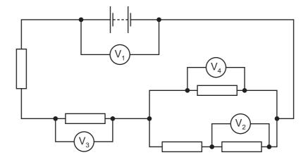
The reading on voltmeter  $V_1$  is  $8.0\,V$  and the reading on voltmeter  $V_2$  is  $1.0\,V$ .
