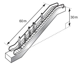
To drive the escalator against the forces of friction when there are no passengers requires a power of 2.0 kW.
