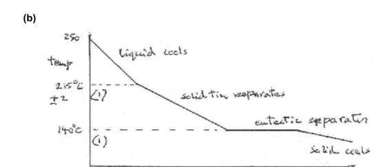
Shape of cooling curve to 140°C (ecf from candidate's graph) (1)
