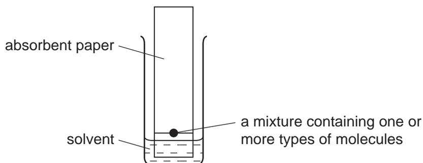
As the solvent rises up the paper, the molecules with the greatest solubility in the solvent travel a fixed distance up the paper. When the solvent reaches the top of the paper, the paper is removed, dried and sprayed with a dye. The different molecules appear as coloured spots.
