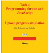
You will notice that when the Upload button is pressed the bar appears to fill in 8 steps using the images Bar1.png to Bar8.png
