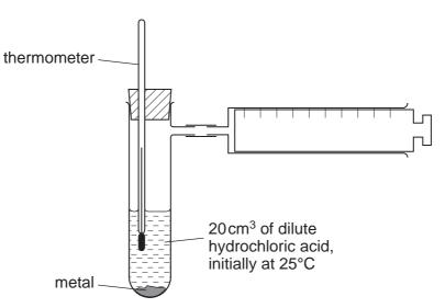
Four metals were used, calcium, magnesium, iron and zinc. In each experiment, the initial temperature of the acid was 25°C.
