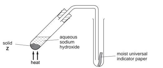
When the tube was heated, the indicator paper turned blue. Suggest the identity of Z.
