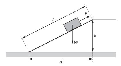
How much work is done in pulling the block up the slope?
