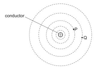
The current in the conductor is into the plane of the diagram.
