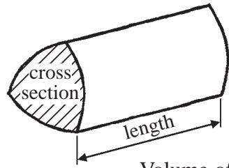
$$\text{Volume of prism} = \text{area of cross section} \times \text{length}$$
