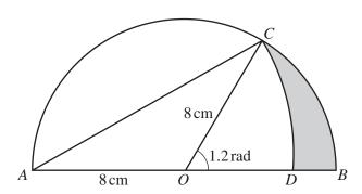
The diagram shows a semicircle, centre O, of radius 8 cm. The radius OC makes an angle of 1.2 radians with the radius OB. The arc CD of a circle has centre A and the point D lies on OB. Find the area of
