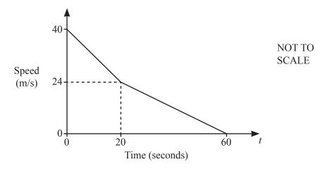
The train slows down uniformly from a speed of 40 m/s to a speed of 24 m/s in a time of 20 seconds. It then slows down uniformly for a further 40 seconds, until it stops.
