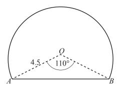
The cross-section of the tunnel is a major segment of a circle, centre O. The radius of the circle is  $4.5 \,\mathrm{m}$  and  $A\hat{O}B = 110^{\circ}$ .
