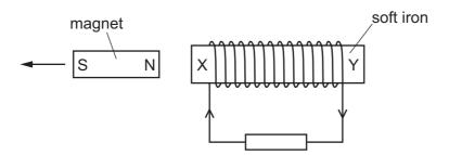
The N pole of a bar magnet is pulled away from end X which causes an induced current in the coil.
