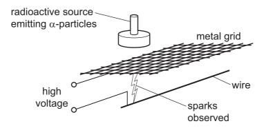
When the radioactive source is placed close to the grid, sparks are observed in the position indicated.
