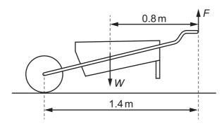
Which vertical force *F* is needed to support the wheelbarrow in the position shown?
