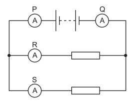
Which two ammeters read the largest current?
