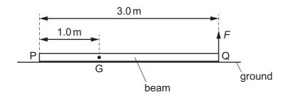
The length of the beam is 3.0 m and its weight is 600 N.
