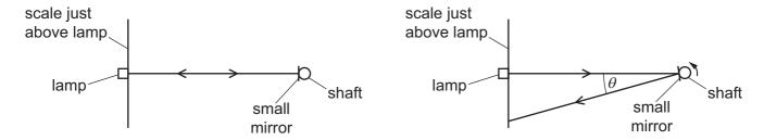
The beam from the lamp reflects from the mirror to give a small spot of light on a scale placed just above the lamp. The shaft and mirror rotate through 1°. The spot of light moves along the scale.
