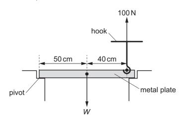
An upward force of 100 N is needed to lift the metal plate about the pivot, as shown.
