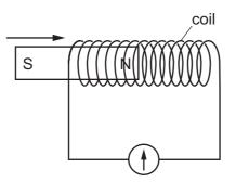
The needle of the galvanometer moves.
