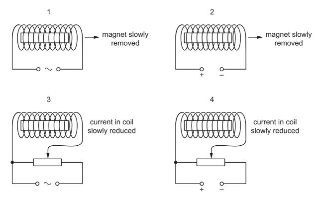
In which experiments is the magnet demagnetised?
