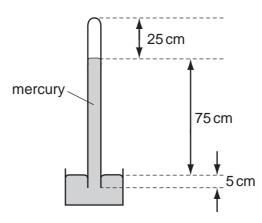
Which distance is used to calculate the pressure of the atmosphere?
