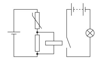
Which change in the environment causes the lamp to be switched on?
