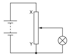
What happens to the brightness of the lamp and the potential difference (p.d.) across the lamp, when the slider is moved from X to Y?
