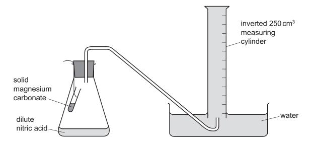
50 cm<sup>3</sup> of dilute nitric acid was added to the conical flask. The contents of the test-tube were released, allowing the solid magnesium carbonate to mix with the dilute nitric acid. A stop-clock was started and the volume of gas collected in the inverted measuring cylinder was measured every 10 seconds for 80 seconds.
