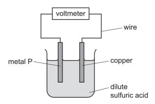
Which metal P produces the smallest voltage?
